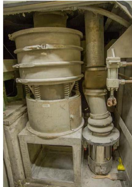
*Figure 3. Sand Separator and Slag Collection Chute*
